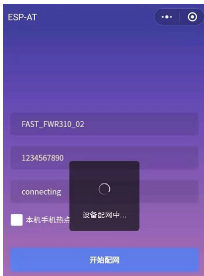
Fig. 16: Connection to the Router via the Applet
